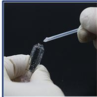
Use the spatula to insert the suspect material into the ampoule
