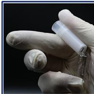
Take the top of the ampoule between the thumb and index finger and snap off the top with the ampoule breaker
